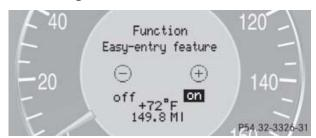
► Press button → or → to switch Function Easy-entry feature on or off.
