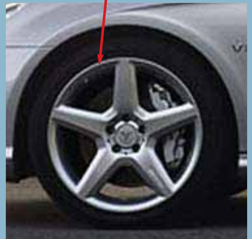
New AMG 19" 5-spoke lightweight alloy wheels (standard) with high-performance tires (Front: 255/35 R19, Rear: 285/30 R19)
