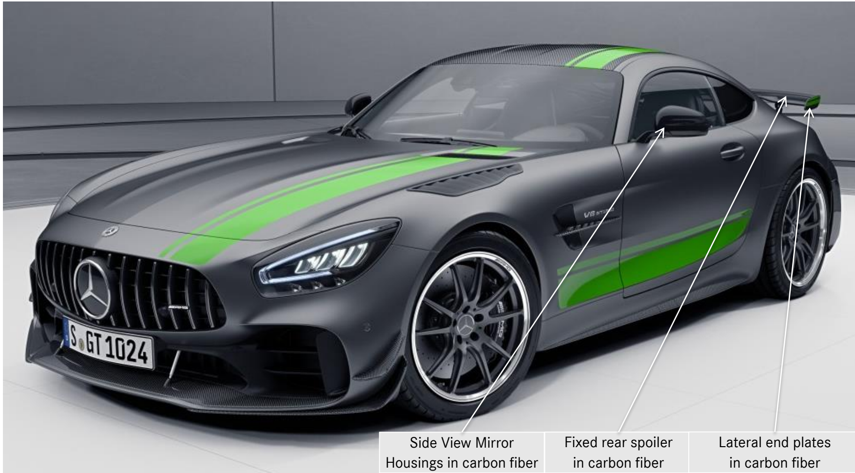
AMG Exterior Carbon Fiber Package II (DC4) Standard on GT R PRO
