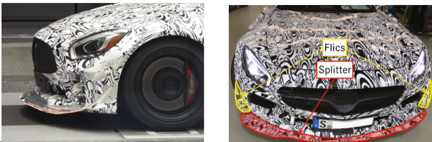
Fig. 6. Splitter proportions and flics to generate similar front lift (FL) as the active aero system on the underbody
