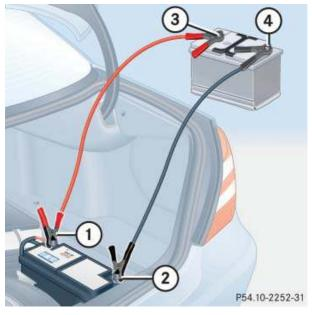
(1) Positive terminal of discharged battery
