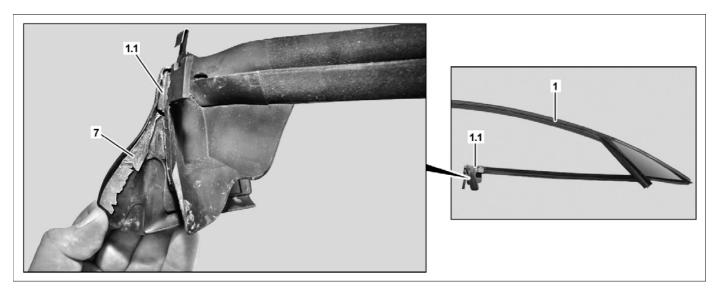
**i** The following work instructions apply for reinstallation of the old sealing profile (1) (on model 207.3) or old sealing rail (on model 207.4).
