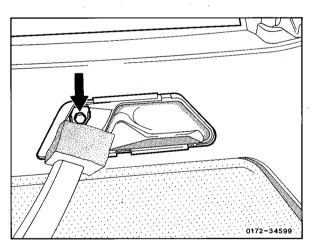
6 Push housing of inside door opener forward and remove from inside door plate.
