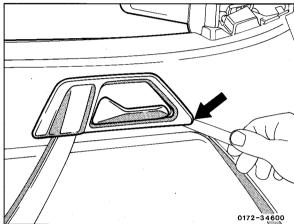
5 Partially pull out foam insert and unscrew screw located underneath.
