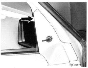
3 Force off molding on inside door actuation and turn out screw inside on handle.
