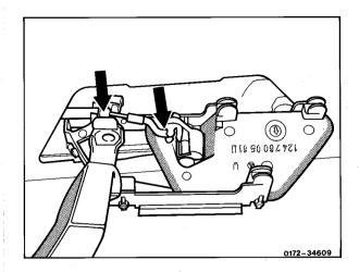
8 Push door lining in upward direction and remove.
