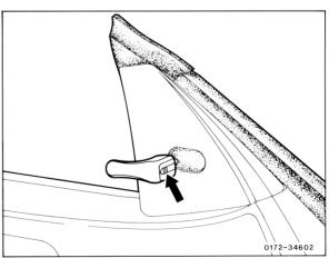
3 Remove covering on door frame from clips and pull out in upward direction.
