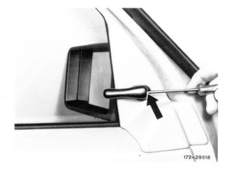
2 Unclip cover at top from door frame and pull out in upward direction.
