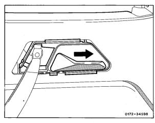
7 Disengage actuating puller on door opener and disengage housing, remove housing.
