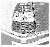
To replace taillamp bulbs, open tailgate and press the clips of the lamp carrier together and remove.
