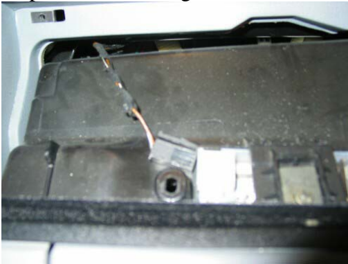
Step4: Disengage cover plate by moving a plastic clip up
