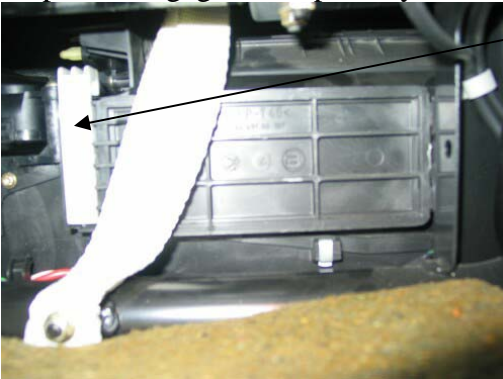
Step4: Disengage cover plate by moving a plastic clip up
