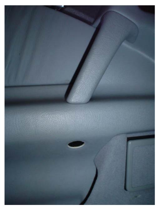
The final one holds the door latch frame onto the panel. Set the frame and screw aside.
