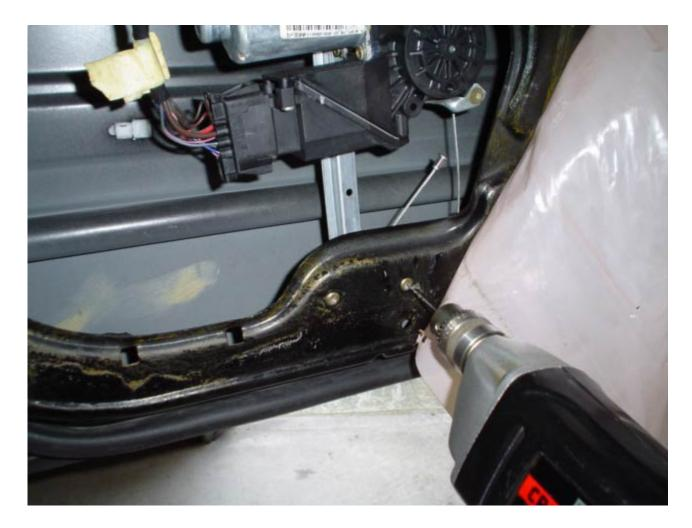
The way it works is that you'll move up a few fractions of an inch on each bit, until eventually the rivet will fall apart into two pieces. No more rivets, just holes:
