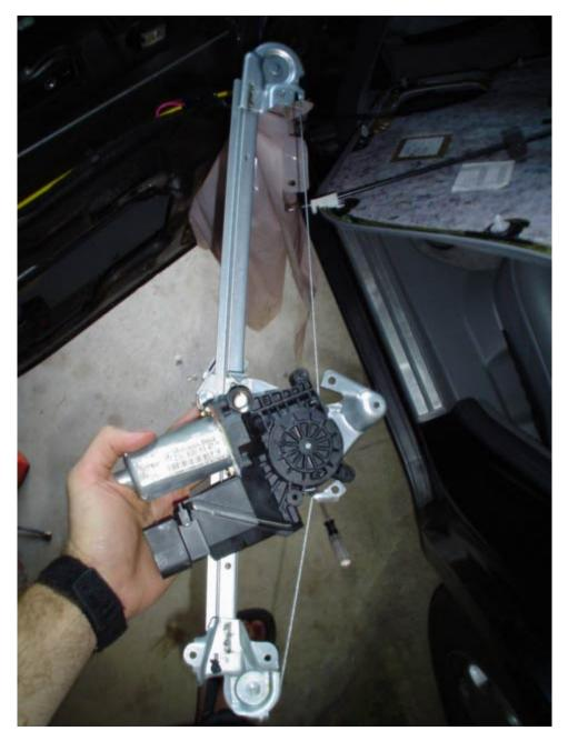
Be sure you've removed all the broken junk from the bottom of the door shell unless you want it rattling around in there. Now remove the tape from the window and pull it down until you can access the rail that holds the glass. Position the new regulator so that it
