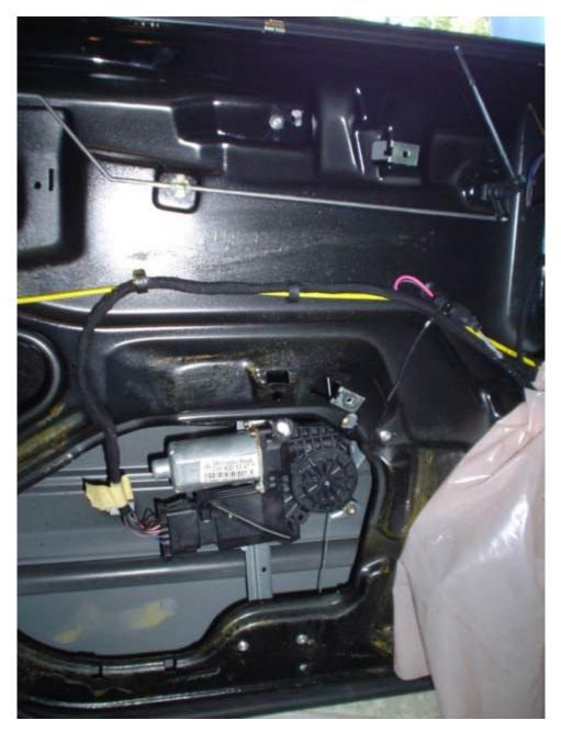
Now hook the motor back up and we need to re-adapt the window. With the ignition key in the 2nd position, move the window up (to the stop) and hold for 5 seconds. Do the same with the down position. Your motor should now "know" the new full-up and full-down points.
