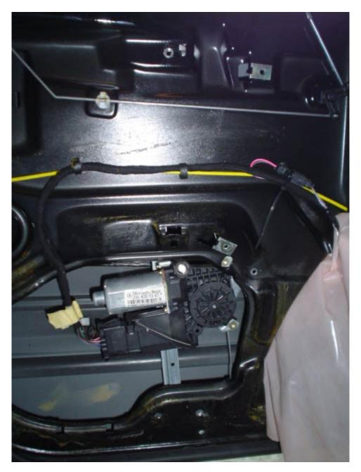
Do the same process with the top two rivets and the entire regulator and motor will come out in a single piece. Make sure you unplug the motor's wiring harness before you pull the assembly out of the door.
