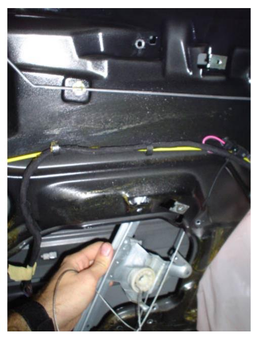
Remove the 2-3 torx screws holding the motor to the regulator. Swivel the motor out of it's spot and rotate it into place in the new regulator. It has a toothed cog that you have to line up. You'll know it's right when you feel it--a very secure connection.
