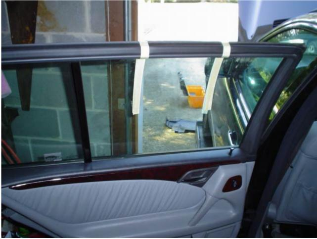
Now let's start the door panel removal by removing three simple phillips-head screws. The first one is accessed by gently prying the door handle liner away from the door. Set it aside.
