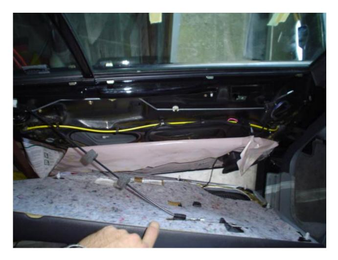
You'll need to first unplug the wiring harness that connects to the window button. Then, pull the door handle and work the cable hook free from the latch mechanism. You'll have to snap the white guide piece free to allow the door panel to pull away:
