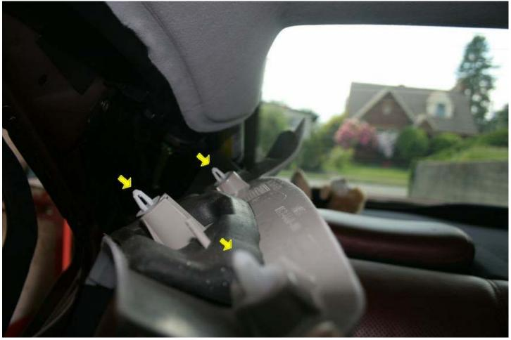
unsnap the little swing up doors in the grab rail to expose mounting screw. 2 screws for each grab rail
