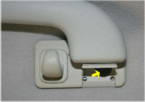
as you peer behind the C-pillar panel you unsnapped, you'll see that the lower corner of the rear of the headliner is secured by a rivet. drill this out. BE CAREFUL ..... that the drill bit doesn't grab the headliner fabric and tear. Can you say "I'll be careful"? I know that you can.
