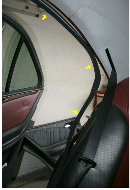
using your fingers, work them into the panel just below the headliner and firmly pull out. the three snaps will give way to expose the bottem edge of the headliner
