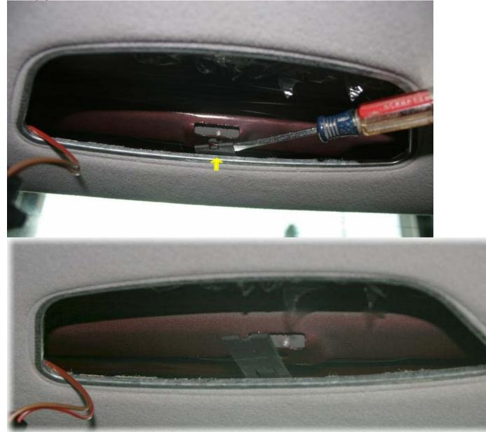
Now, repeat on other side: pry off door weather stripping, removal of other grab rail, pop open C-pillar liner, and drill out rivet.
