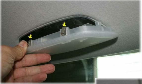
disconnect wiring connector and set light aside
