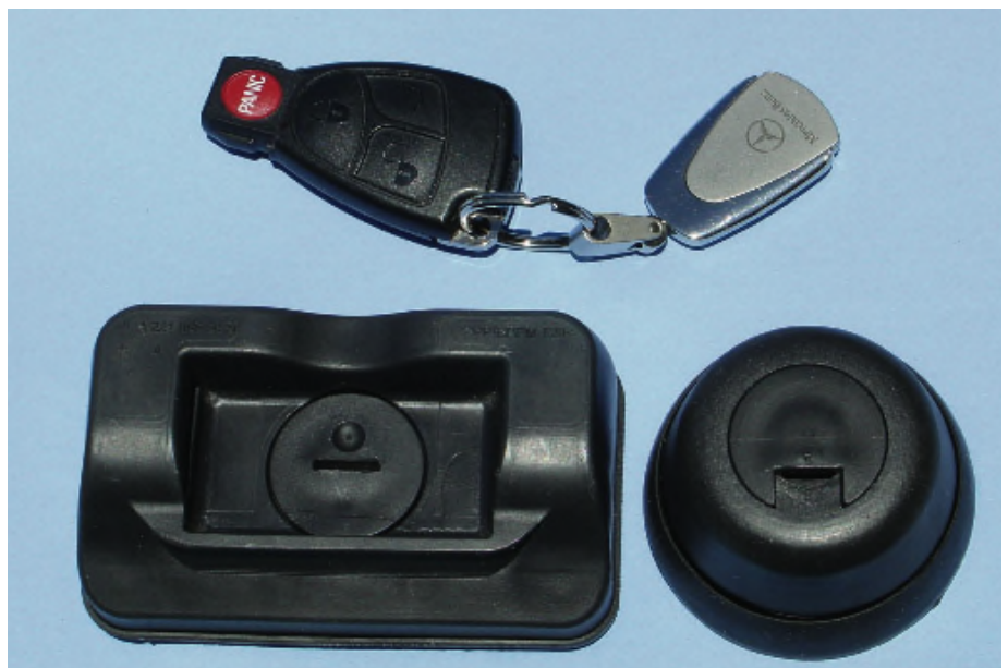
Typical jack point along side skirts of late model (left 221-998-00-50) and previous generation (right 002-997-06-86) M-Bs.
