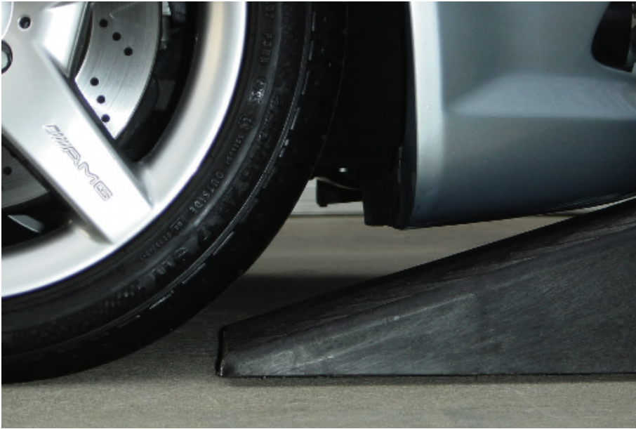
Popular automotive ramps typically will not work with MB cars equipped with AMG front bumpers.
