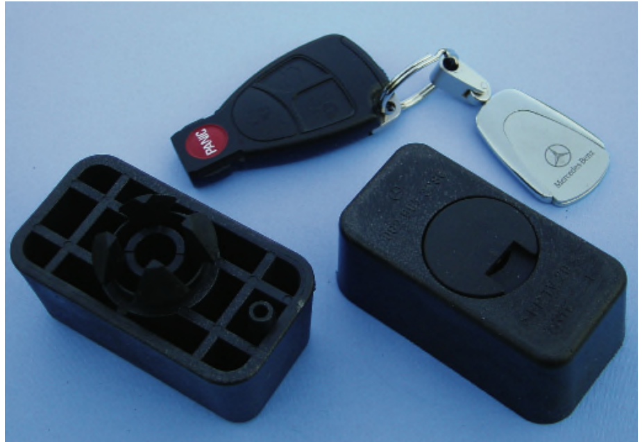
Top and bottom view of W211 engine cross-member jack point, PN 002-997-32-86.
