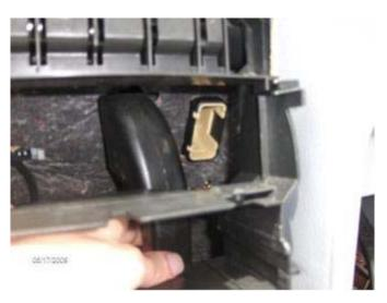
Just yank it off and then twist it out. Pictured above is the passenger's side duct work. It's not held on by anything other than friction. The driver's side takes a bit to twist out. I just about folded it to get it out. The tubing will snap back into shape.
