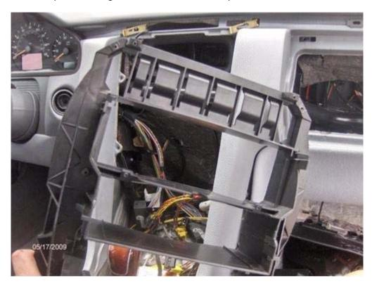
To install the double din, pretty much do everything in reverse. The main thing to remember is to install the ac/heat duck work on just the driver's side before you put the double din cage in place. The driver's side has less wiggle room, and doing this first is the only way I could get the duct work attached properly.
