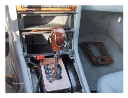
You will want to remove the molding and compartment of the lower console just as the video shows. I did it later in the process, good idea to get it done right away.
