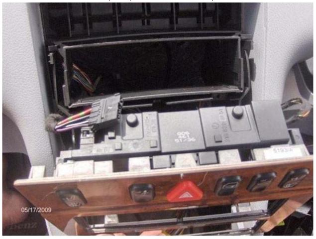
The trim is held on by 2 black screws under the climate control unit. After these are gone, the trim panel will be sitting in your hand. The switches will still be attached to the back of the burlwood.
