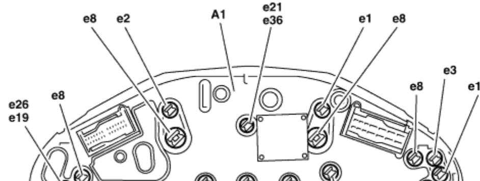
e19 Catalytic converter overheat warning lamp
