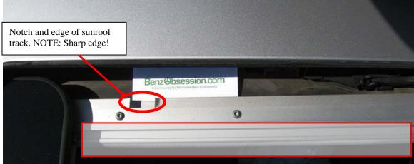
The area in the shaded box in the picture above is the track for the sunroof liner (sunshade). This should be wiped clean of any dirt or debris, but does not need special lubrication.
