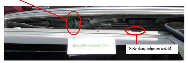
Getting the grease into the groove can be a bit messy. After some experimentation I found that putting a small amount right down into the notch and then operating the sunroof a couple of times distributed it along the groove. You could try applying it with the allen key, but it is quite hard to see into the groove to see how well you are doing.
