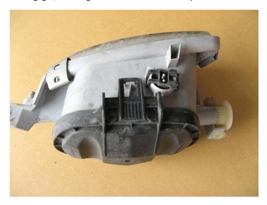
Access door opened -- the bulb for this light broke off at its base when I tried to remove it from the connector. The connector was melted to the bulb (see below).
