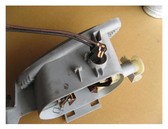
And, snapping the grommet into the housing. This grommet seemed to want to snap one way and not the other. What I noticed about this is that when it snapped in correctly, the connectors on the wires were lined up perfectly with the bulb.
