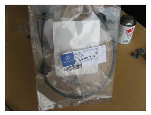
This is the harness itself. At the top of the picture is the two-pole, female connector, which snaps into your existing harness. At the bottom center is the 'grommet' which snaps into the foglight housing. At bottom right, the shielded (+) and unshielded (-) connectors for the bulb.
