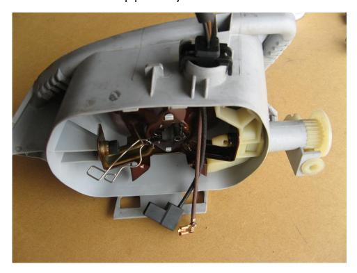
Note that the reflector is actually coated steel. The negative terminal (brown), simply connects to a spade connector built into the reflector housing, just above the bulb spring. The positive connects to the single spade terminal from the bulb.
