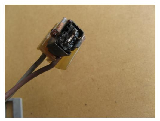
Note that the connector inside the housing is too big to fit through the opening, so I just cut it off.
