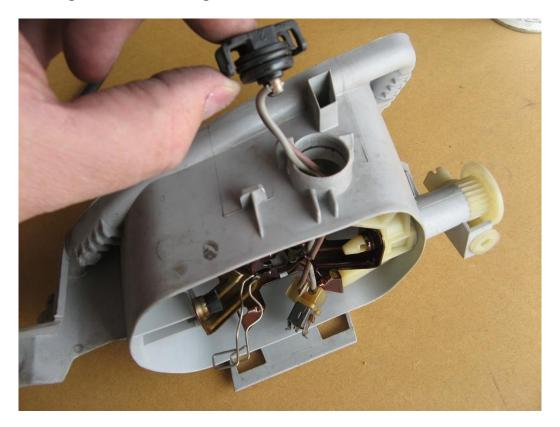
This photo shows how badly the connector was melted to its plastic shield.
