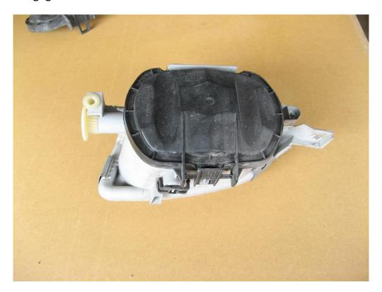
The Bottom of the foglight, showing the connector for the lamp harness.
