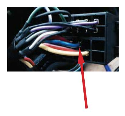
Insert the Blue/White wire next to the Red (Accessory) wire and above the Orange/White (Illumination) wire. Connect the Blue/White wire to the remote turn-on wire on your Pioneer radio.
