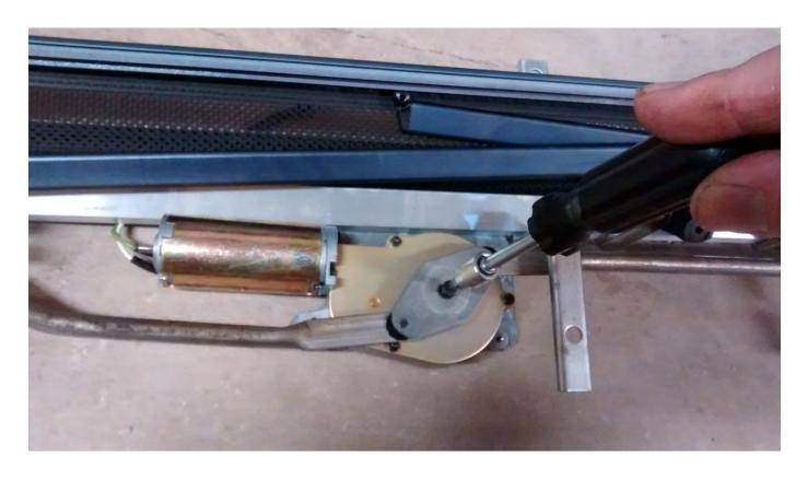
Remove one each shaft Torx bolt to release swing arms. Remove three each Torx bolts to release motor mechanism. NOTE: New mechanism may require an adaptor (included with new part) to fit the original swing arms.
