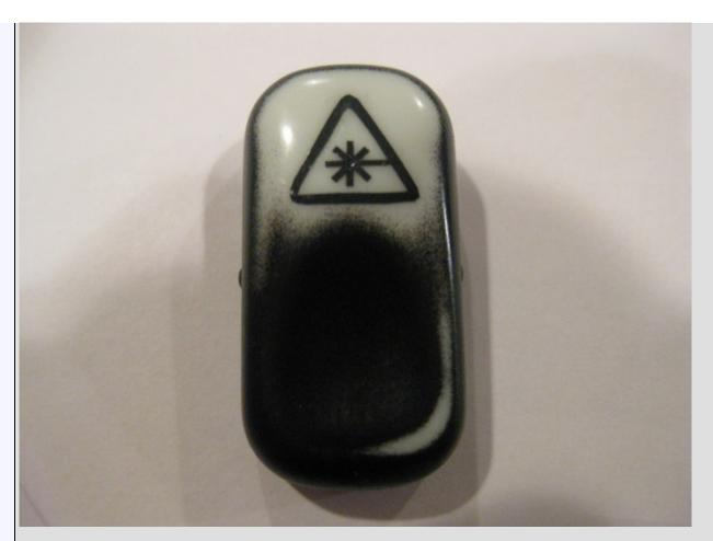
I painted it with Krylon Fusion for plastic in satin black which is almost a perfect match to the original MB finish. After peeling off the masking I was left with a factory looking switch.... After some searching I also located the 4 hole wood trim I needed to add this extra switch.
