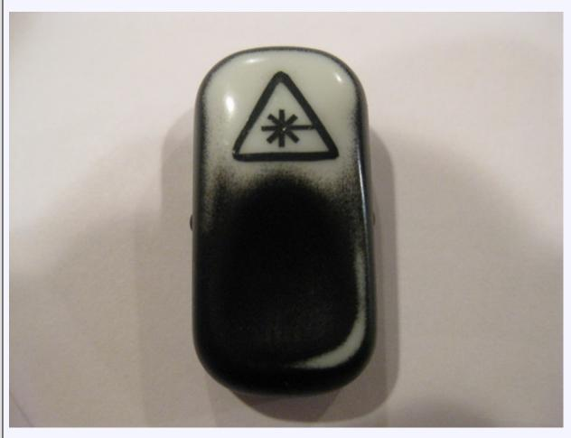
I painted it with Krylon Fusion for plastic in satin black which is almost a perfect match to the original MB finish. After peeling off the masking I was left with a factory looking switch.... After some searching I also located the 4 hole wood trim I needed to add this extra switch.
