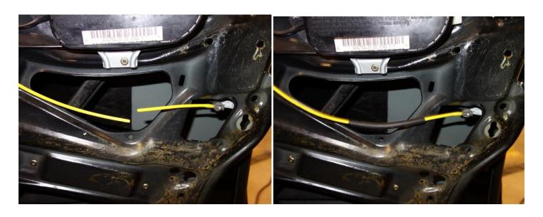
•Drill out two bottom rivets of window guide.
