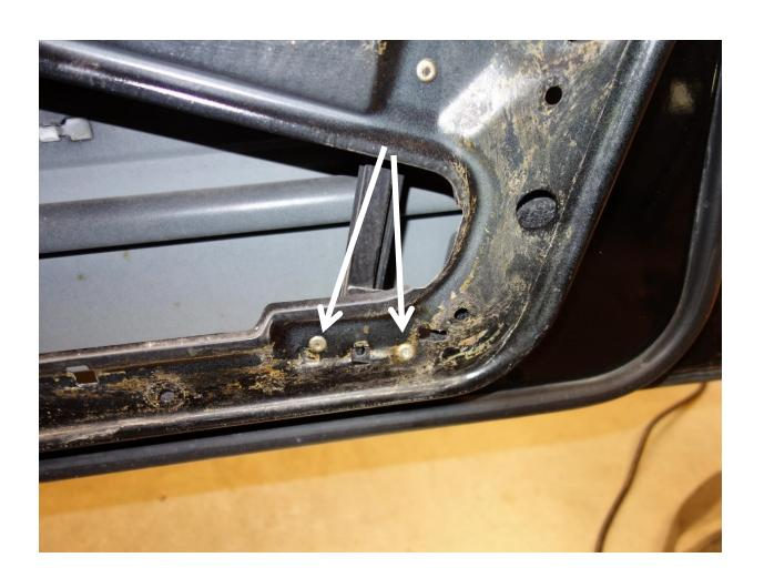
•At top of window guide, drill out rivet closest to the lock assembly.
