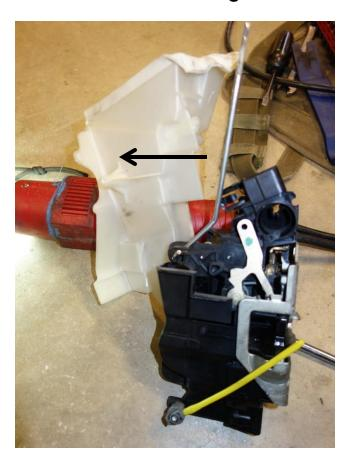
•On the old lock assembly, measure the distance of the release lever from the plastic housing. In this case, ~ 1 & 7/8ths of an inch.
