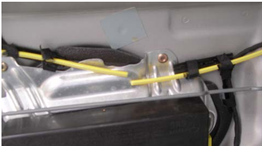
Figure 17 Cut Yellow Vacuum Line
