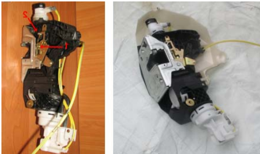
Figure 5 Actuator on Left has Soft/Self Close Feature, Actuator on Right Doesn't
