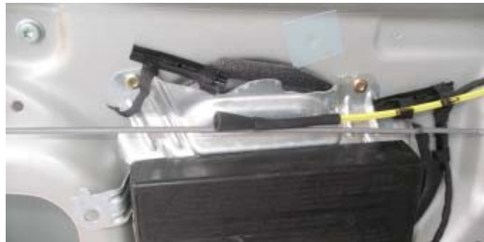
Figure 19 Plugged Vacuum Line
