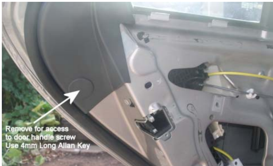
Figure 6 Remove this Plug to gain Access to the Rear Door Handle Screw
