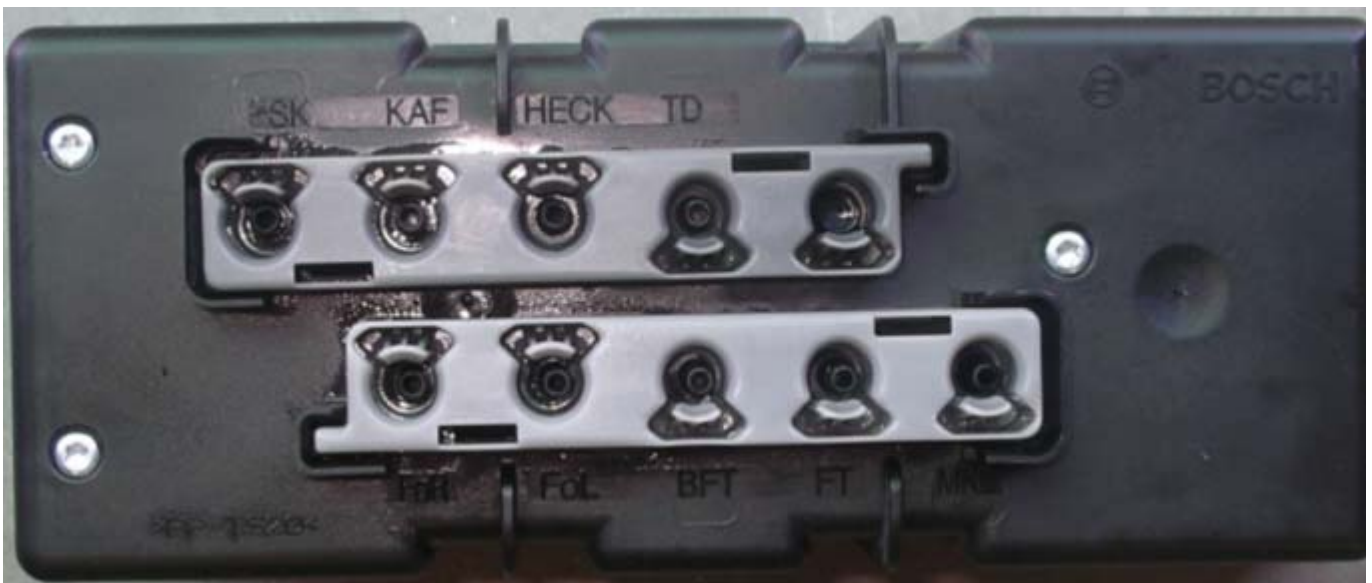
Figure 2 PSE Pump Air Line Port Designations
