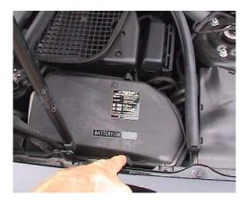
3. Slide the locking tabs to the unlock position on both sides of the cover and then remove the cover. The ECU has five connectors plugged into it.
