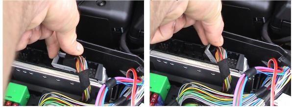
Finish installing the connectors in the reverse order of which they came out.
