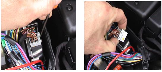
5. Once the outer connectors are removed, the three center connectors must be removed in sequence. Starting with the outermost connector, depress the tab in the center of the connector while sliding the retaining arm downwards in order to remove the connector.
