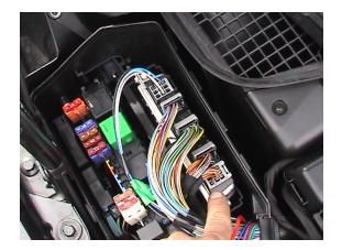
4. You first must remove the two outer connectors before you can remove the inner ones. Warning! Do not pull on the wires. Pull only on the connector itself. To remove the outer connectors, first depress the tab while gently pulling up on the connector.
