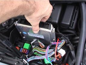
8. Installation of the ECU is done in reverse order. Note: To install the connectors with the retaining clip, just gently place the connector over the proper position with the retaining clip in the downward
