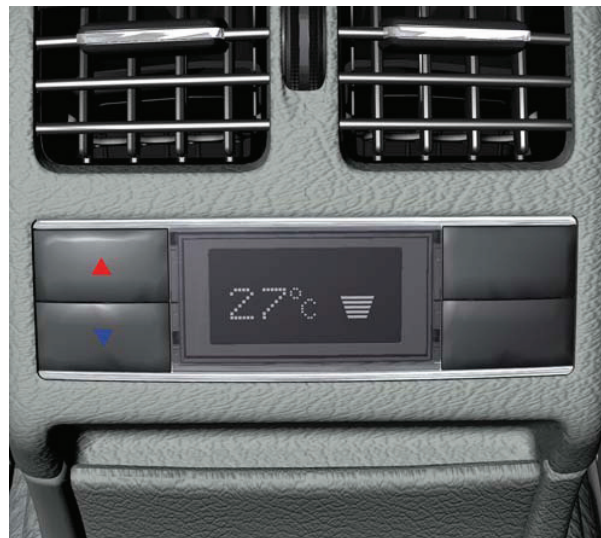
Rear AC operating unit
