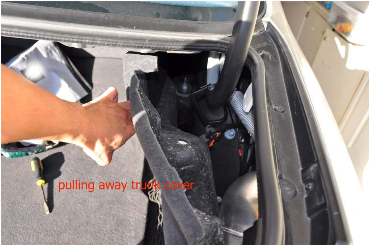
3. Cover is removed, top of the shock absorber is accessible
