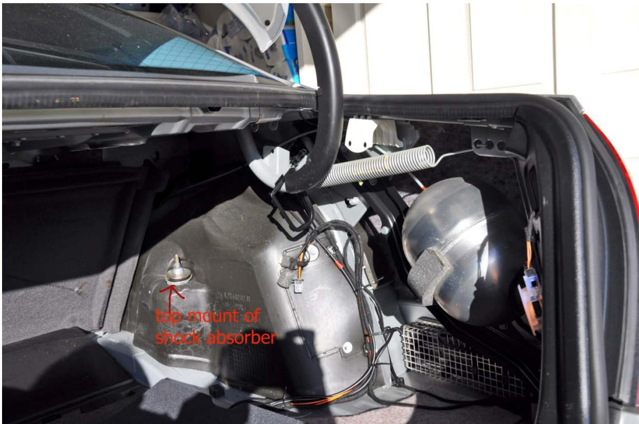
4. Remove the top mounting nut. Put a vise grip on the stub of the shock absorber to prevent it from spinning
