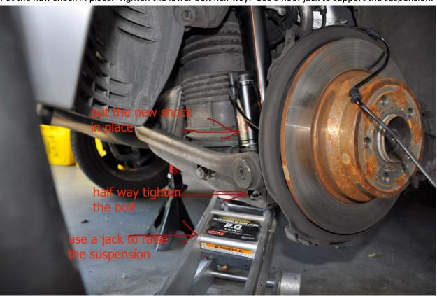
13. Use a floor jack to raise the suspension and align the stub of the shock absorber to the mounting hole and cut the wire. Once the wire is cut, the shock will expand. Tighten the nut on top of the shock. Remove the cut wires.
