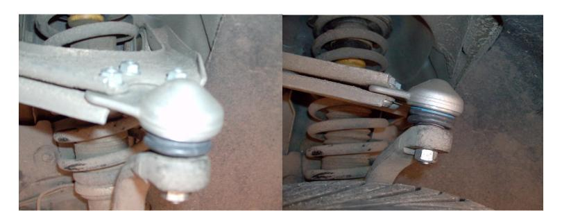
All work can be done in about 30 minutes, the only problem you might face is with removing the ball joint from the steering knuckle.
