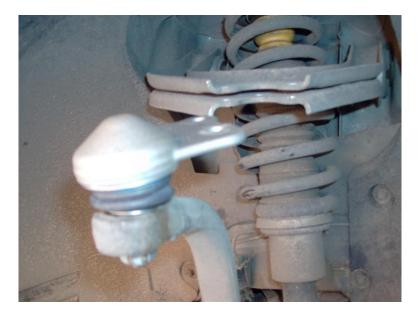
6. Then put the ball joint into the upper control arm and tighten all 3 screws.
