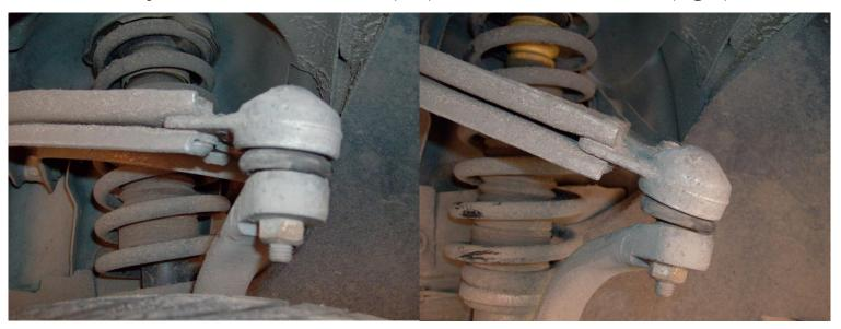
3. We have to remove 3 screws from the upper control arm and one nut from the joint.
