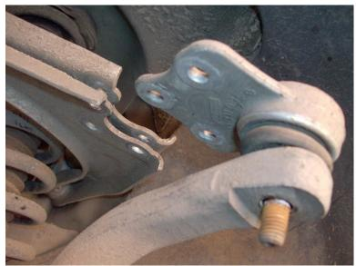
4. Then it's impossible to remove to old ball joint since it was pushed under a pressure. I didn't have a special kit for ball joint, so I had to use a little vise...:) In order to do so, I had to cut the thread.
