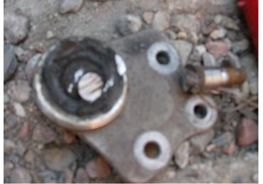
5. Then just put the new ball joint and tighten the nut on the bottom.
