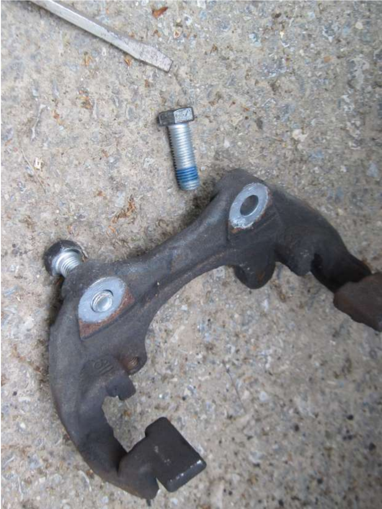
Brake Anchor, with 18mm bolts
