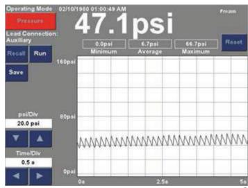
Then, we decide to perform an Engine Mechanical Health Condition Test using the vacuum transducer connected to the intake manifold, so we can see the amount of vacuum created by each engine cylinder. This information is displayed as either a high-resolution waveform or a percent per cylinder bar graph. I prefer the high-resolution waveform (used in this article) because it gives me more information (when a car is having a
