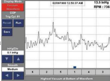
Vacuum is formed by the downward movement of the pistons during the intake stroke. If the cylinder is sealed, a maximum amount will be formed. High vacuum improves volumetric efficiency. A normally running engine produces a uniform amount of vacuum on each cylinder.
