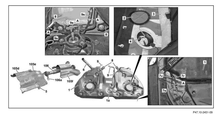
1 Fuel tank 7r Fuel return line 105e Heat shield Nut 7s Connector hose 105f Heat shield 1a 2 Left cap 7v Fuel feed line 106 Propeller shaft З Insulation mat 8 Retaining strap 106a Propeller shaft intermediate 4 Electrical connector 9 Vent line bearing 5 Crossmember 9s Connector hose Α CLIC clamp 6 Filler hose 105d Heat shield
