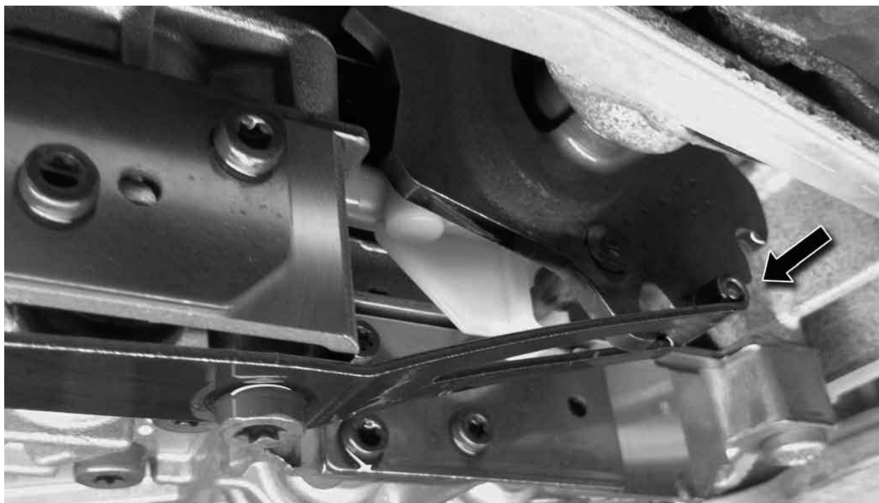
Correctly engaged selector valve in selection range detent plate
