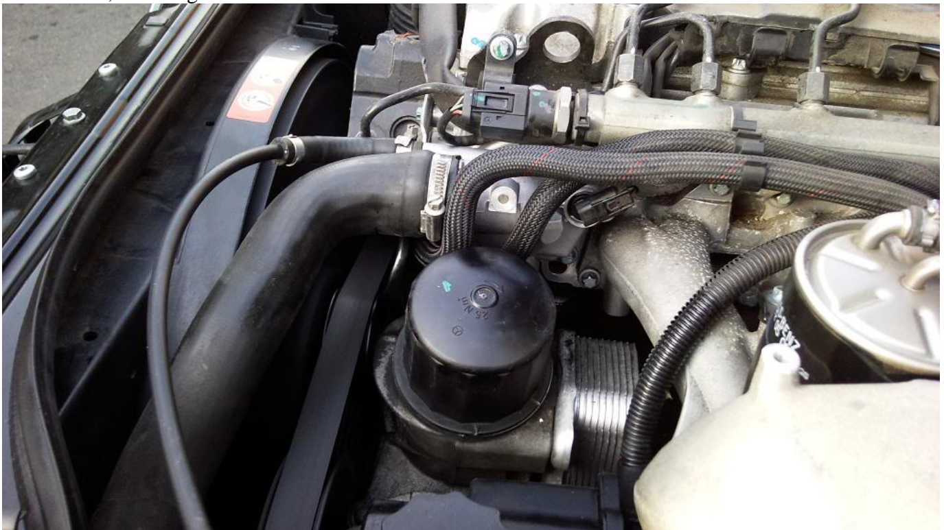
10. Test run, checking for leaks.
