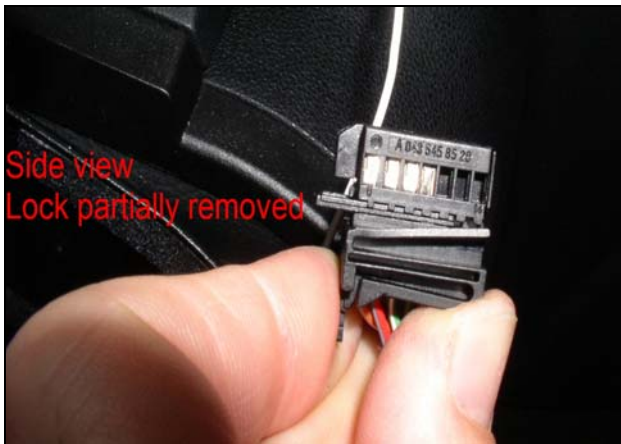
Figure 10 P-B-91.60/99c Slide lock out of connector to remove/install terminals (Repair up to MY 04)
