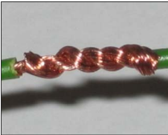
Figure 5 P-B-91.60/99c Wires braided
