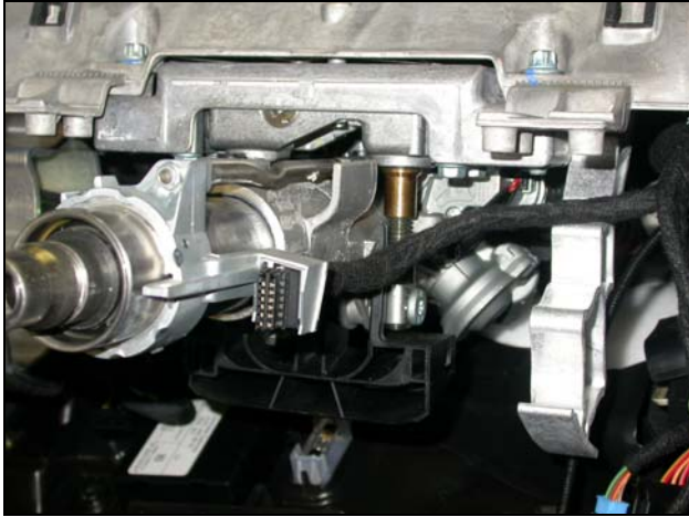
Figure 1 P-B-91.60/99 Harness routing version 1 (approx. length 220mm)
