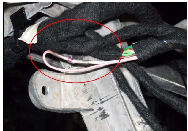
Figure 11 P-B-91.60/99c Repair wire loop. Repeat for all, except steering wheel heater wires. (Repair up to MY 04)
