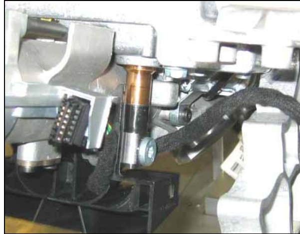
Figure 2 P-B-91.60/99 Harness routing version 2 (approx. length 330mm)
