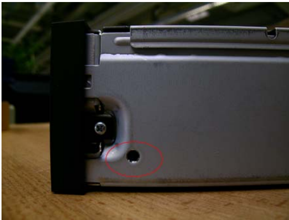
Figure 3 – Bolt is too long P-B-82.64/607
