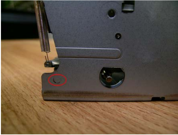
Figure 1 P-B-82.64/607 Shows physical damage to the internal drive
