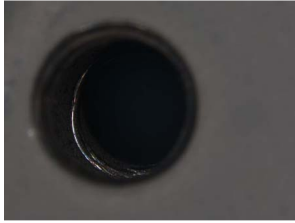
Figure 2 P-B-82.64/607 Close-up of threaded hole with physical damage
