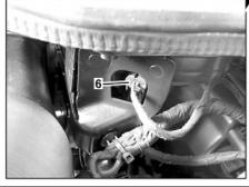
Disconnect/connect ground line on battery
