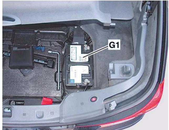
G1 On-board electrical system battery
