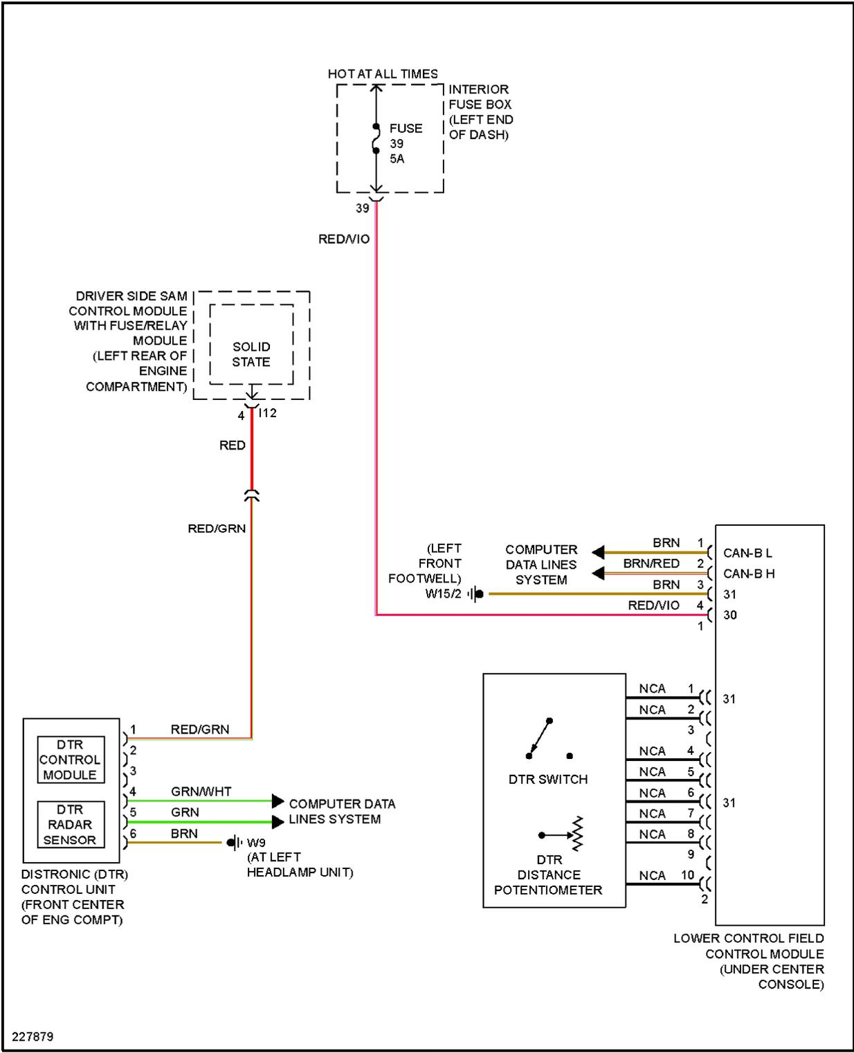
**Fig. 19: Electronic Accelerator/Cruise/Idle Speed Control Circuit, Late Production**
