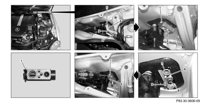
1 Expansion valve 2 Suction pipe 3 Pressure line
