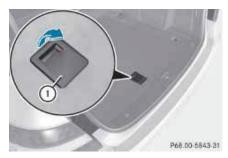
▶ Lift the trunk floor using floor handle (1).
