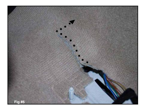
This allows the carpet to fold downward after the insulation is cut away, and the pedal is back in place. The Sprint Booster adds about a 1" to the old connector length, interfering with the carpet if Step 4 and Step 5 are not done. The carpet being more relaxed puts less stress on the connector to avoid failure.
