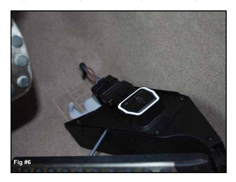
Step 7- Flip the pedal back over and re-secure the pedal to the floor. If you cannot place the pedal back in its original location with slight pressure by hand, then you need to take out more insulation/padding. Your cut in the carpet may also be a bit short. Once you feel this fitment is good, re-attach the pedal as shown in Fig # 1
