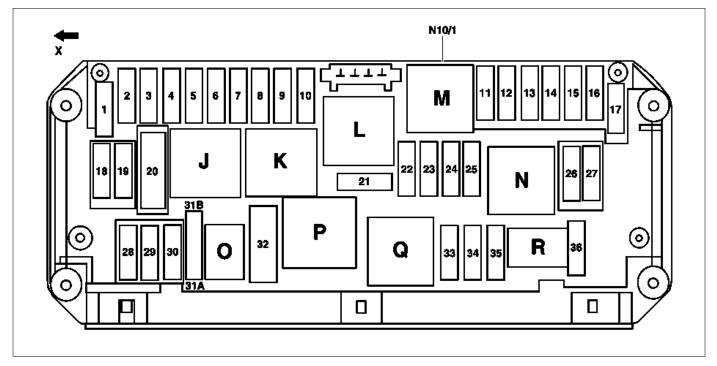
N10/1 Front SAM control unit with fuse X Direction of travel and relay module
