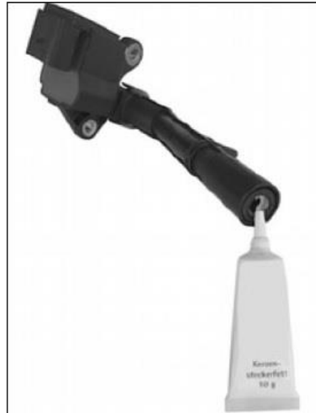
Figure 1. Applying grease. P15.10-2553-02
