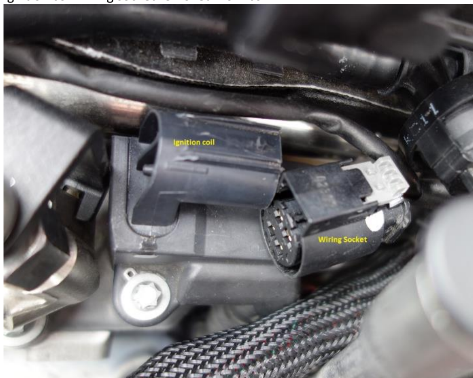
Ignition coil wiring socket removed from coil:
