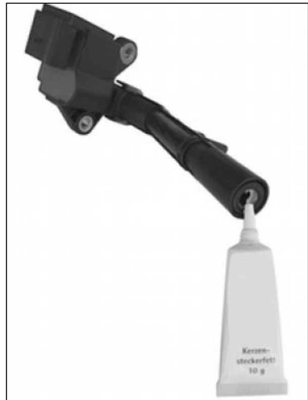
Figure 1. Applying grease. P15.10-2553-02
