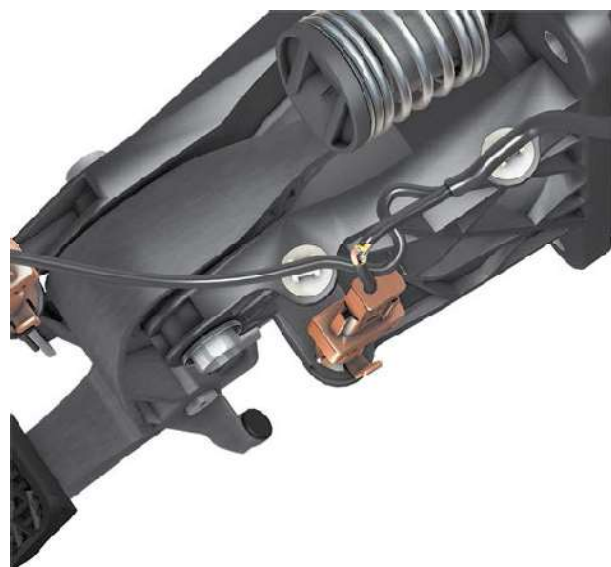
Damage to the electrical feed lines of the clutch pedal switch
