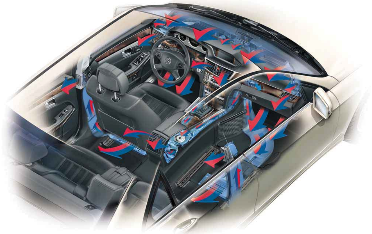
Interior climate control air outlets
