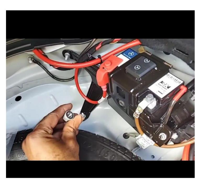
There were two existing ground posts. The one I used for my Amp (-) was unused. It was probably for cars with full size battery in the trunk. The one on the opposite side(not pictured), is attached to the negative cable for my auxiliary battery. I decided to use the one pictured because my ground cable would have been too short to hide wiring behind sub if I used the other.
