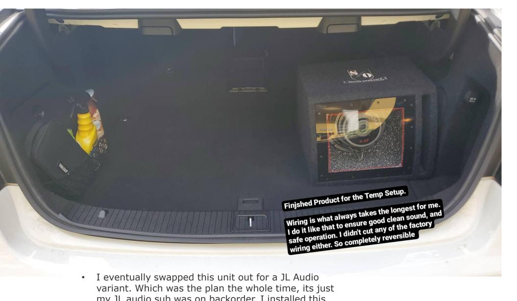
• I eventually swapped this unit out for a JL Audio variant. Which was the plan the whole time, its just my JL audio sub was on backorder. I installed this because driving around with no bass was driving me nuts. Especially after going from my BMW F10 HK logic7 sound system (Excellent), to the Mercedes Variant (4/10 in my audiophile opinion).
