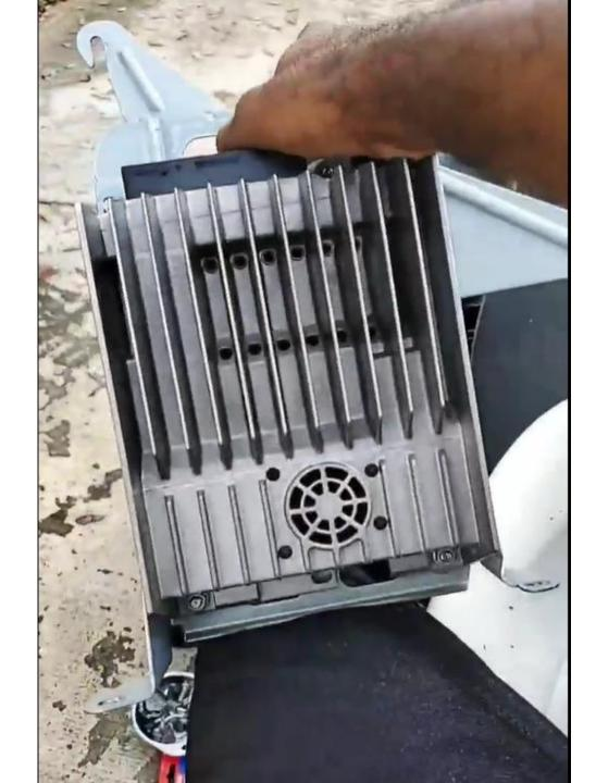
Amp secured to Amp mount by 4 10mm screws. I didn't see the ones on the bottom so I just removed the whole mount.
