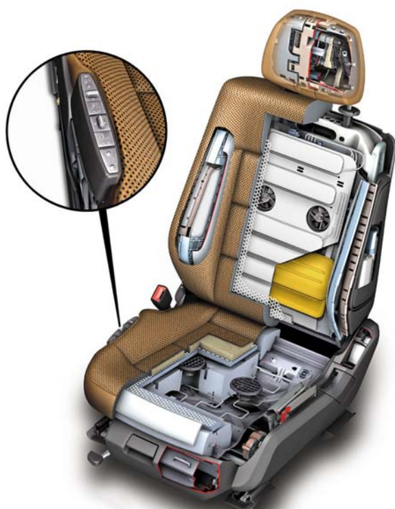
Sectional view of active multicontour seat
