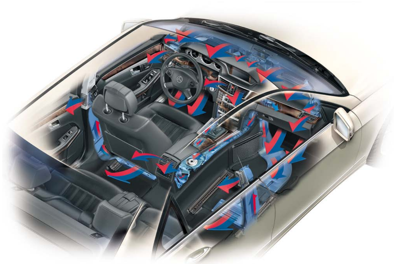
Interior climate control air outlets
