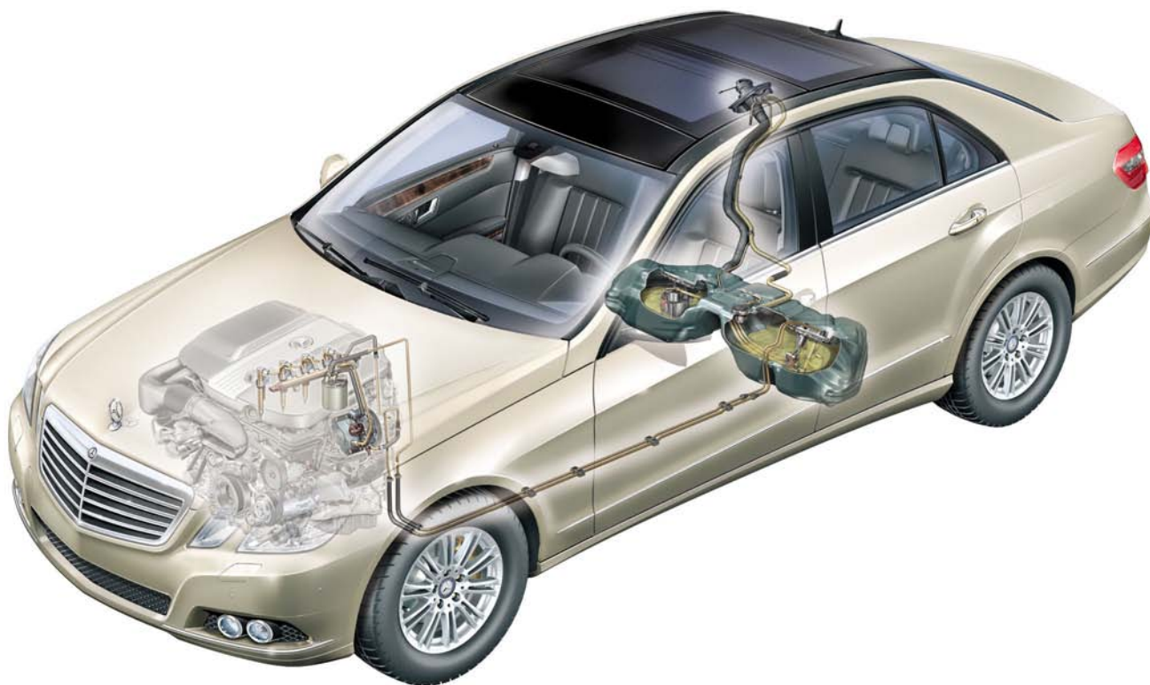
Fuel system in E 250 CDI with OM 651
