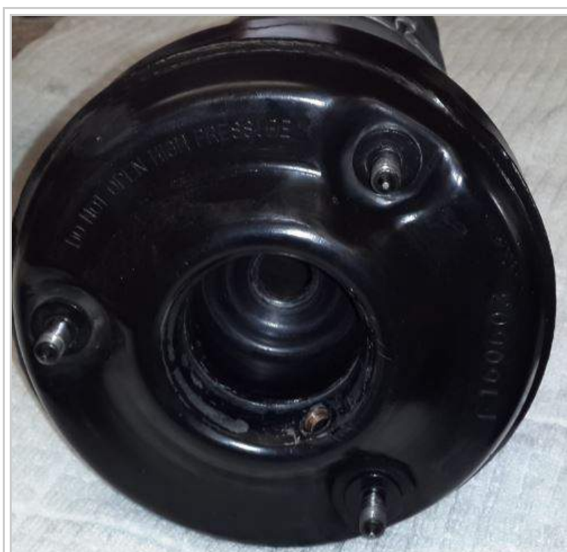
Outside view of the strut with bush removed.
