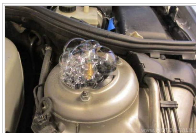
Front strut top seal leaking.
