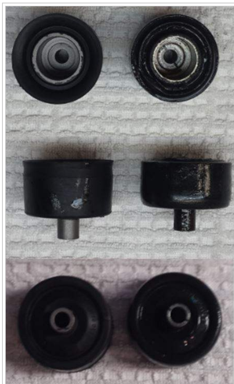
Top bushing: new (left) vs old (right). Note the difference in height in the side view.
