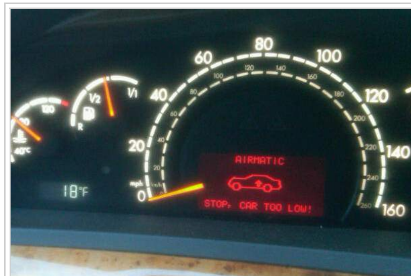
"AIRMATIC STOP, CAR TOO LOW!" warning on the instrument cluster.
