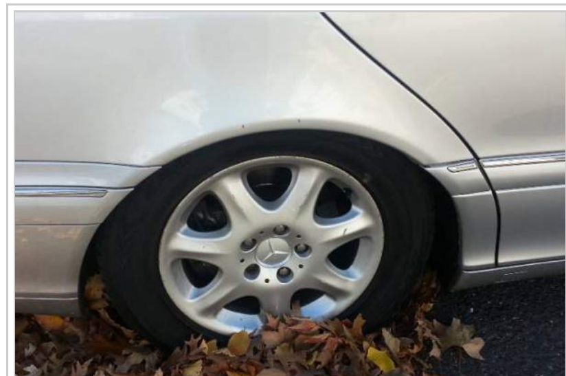
Airmatic strut with too low pressure resulting in vehicle height being too low.
