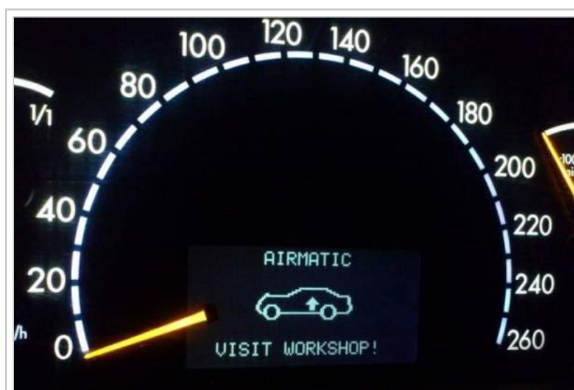
"AIRMATIC VISIT WORKSHOP!" warning on the instrument cluster (facelift).
