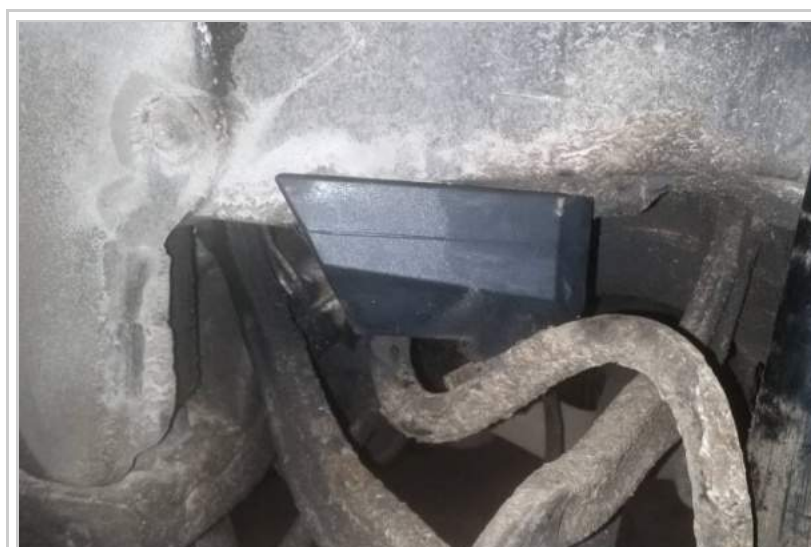
Rear limp-home buffer (installed).
