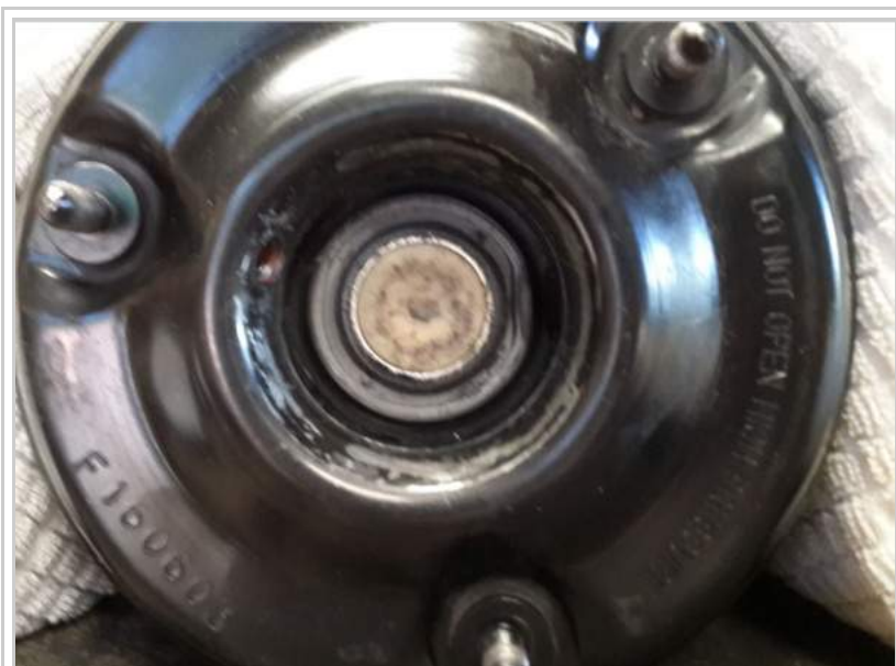
Strut after removing metal disc.
