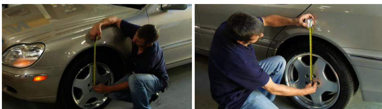
Sample results with no AIRmatic leaks.
