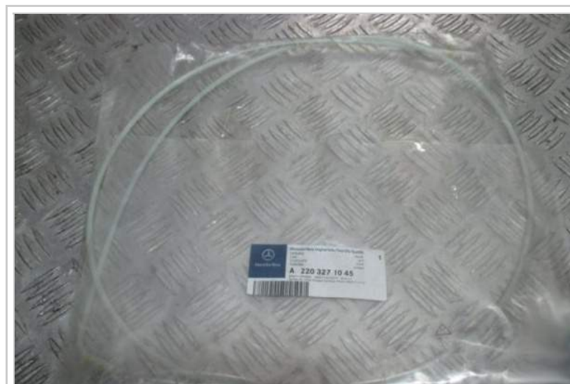
Repair section of air line (A2203271045). Price EUR 14.
