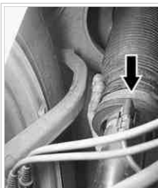
Picture 3: Pull the air spring plunger downwards by hand and press on bearing.
