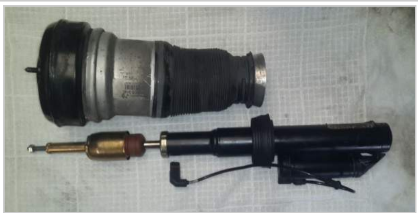
Strut spring separated from damper unit.
