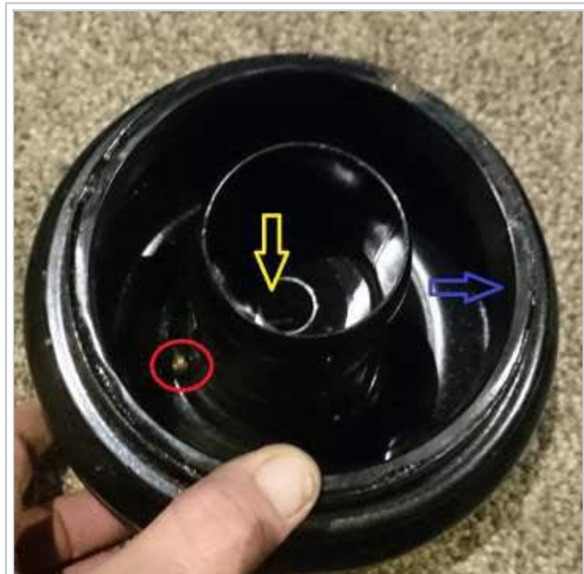
Inside view of the strut with bush removed.
