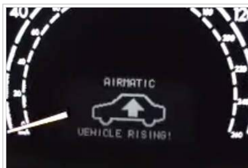
"AIRMATIC VEHICLE RISING!" message on the instrument cluster (pre-facelift).
