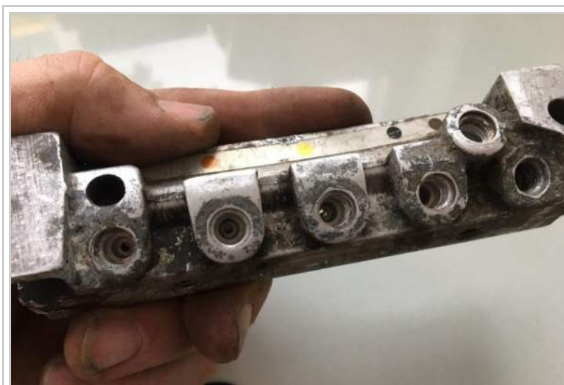
Oxidation in ports
