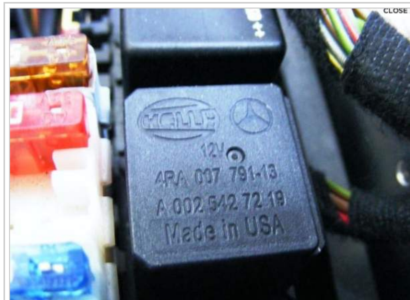
Airmatic compressor relay (A0025427219).
