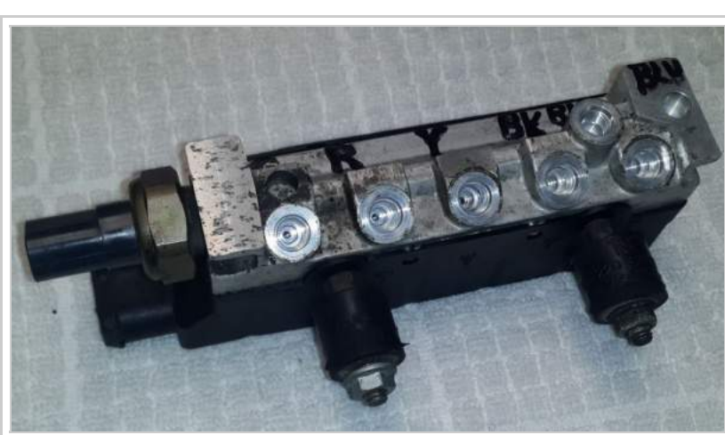
Valve block with lines removed.
