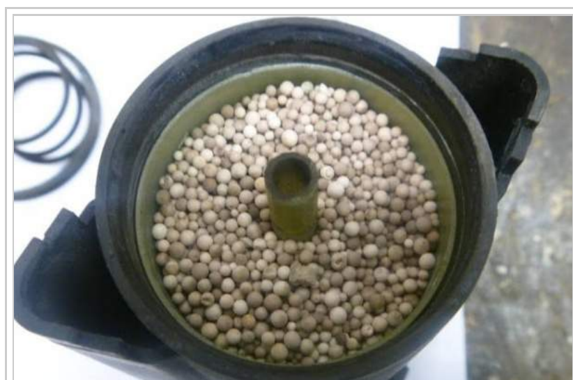
Air dryer desiccant - silica gel.
