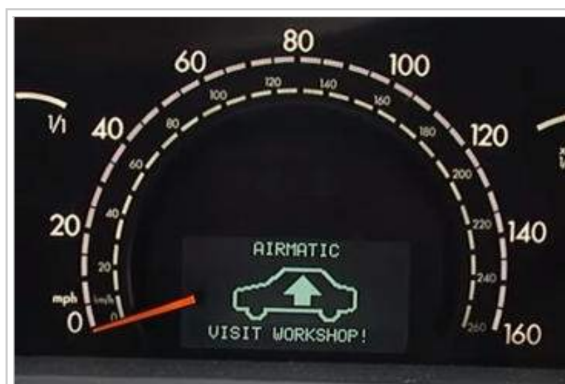
"AIRMATIC VISIT WORKSHOP!" warning on the instrument cluster (pre-facelift).
