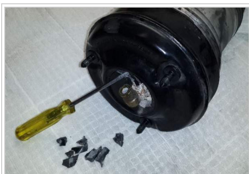
Removing top seal of front strut.
