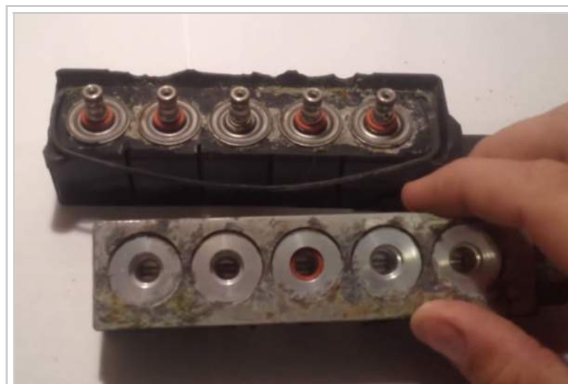
Oxidation between block halves
