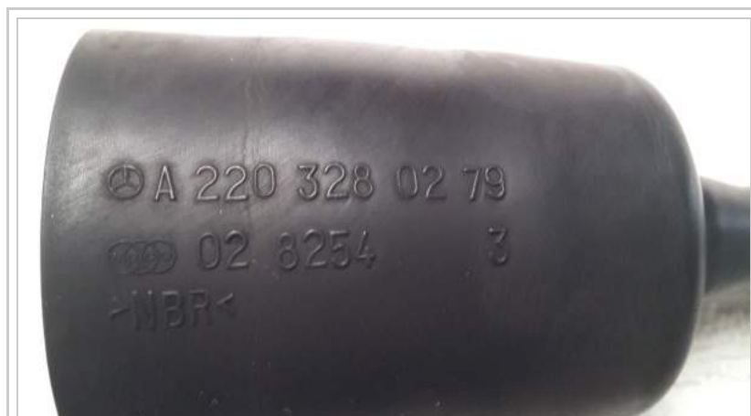
Air filter protective boot (facelift A2203280279, pre-facelift A2203280179).
