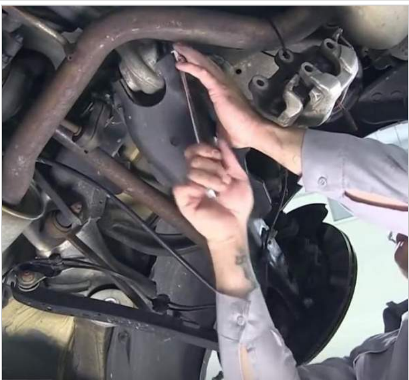
Loosening the inner bolted connection of spring control arm to axle carrier.
