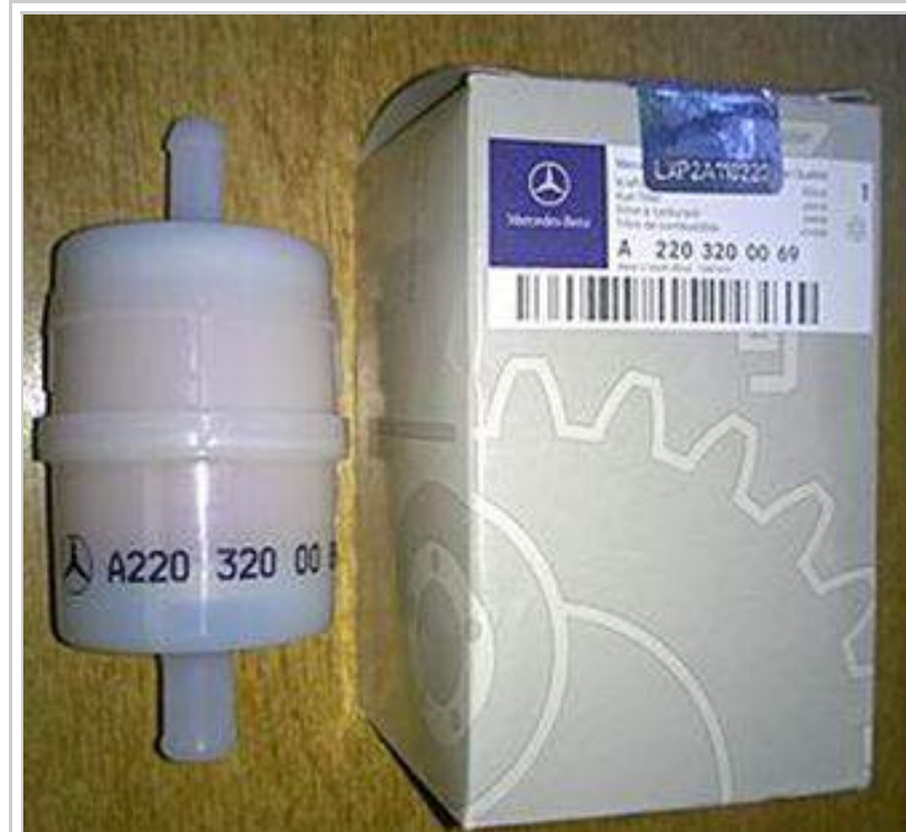
Airmatic air filter A2203200069 (OEM MANN part: WK 32/6).
