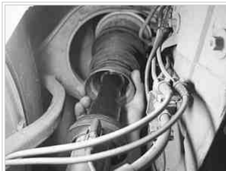
Picture 2: Grasp the air spring plunger (7) with the hand.
