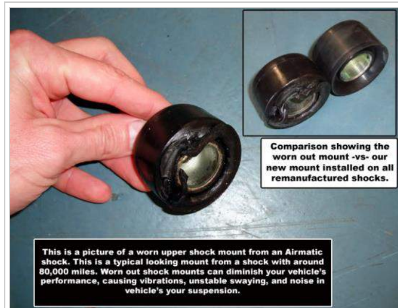
Worn upper mount rubber bushing.
