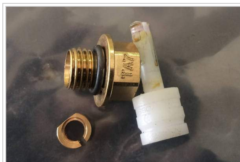
Connector to connect air hose to struts, reservoir and valve block (A0003270369). Price EUR 4.
