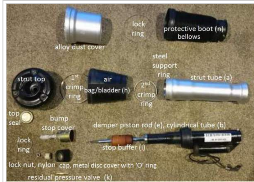
Components of front axle spring strut.
