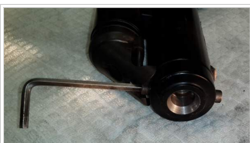
Strut with stub screws partially unscrewed.
