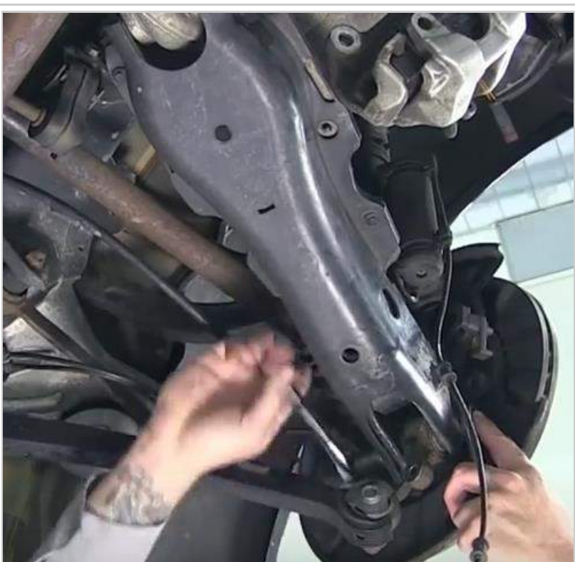
Undoing spring control arm to wheel carrier bolted connection.
