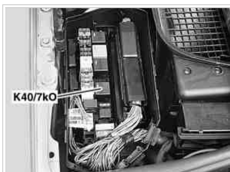
Airmatic compressor relay in fuse box.
