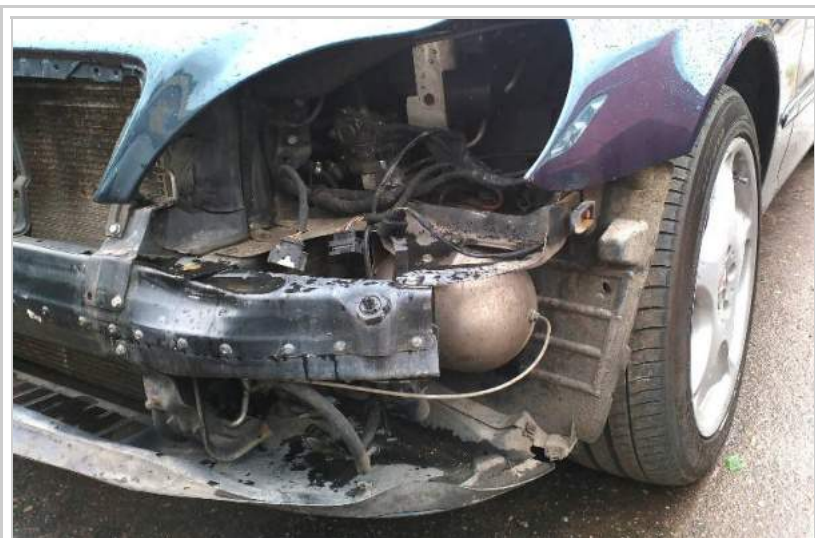
AIRmatic central reservoir shown with bumper removed.
