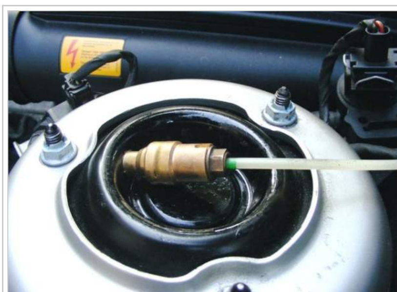
Oldest style front strut without epoxy.
