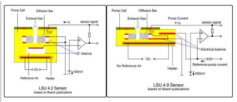
LSU 4.9 gets rid of the reference air, and therefore gets rid of the biggest failure mode. As a result, LSU 4.9 has a long life and can maintain the accuracy throughout the life. Only since then, Bosch LSU sensors have been used widely in the auto industries.
