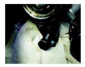
Fasten the special tool - Installer W276 589 00 33 00 to threaded holes of the chain tensioner.
