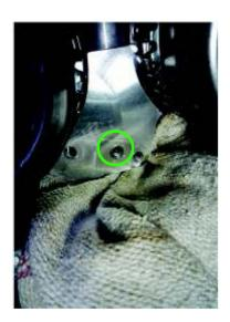
Ensure that the check valve is flush with the cylinder head surface - after installation.
