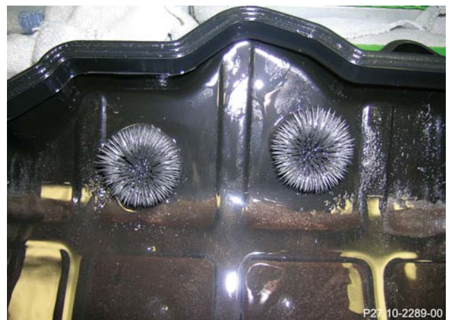
Oil pan with significant wear debris
