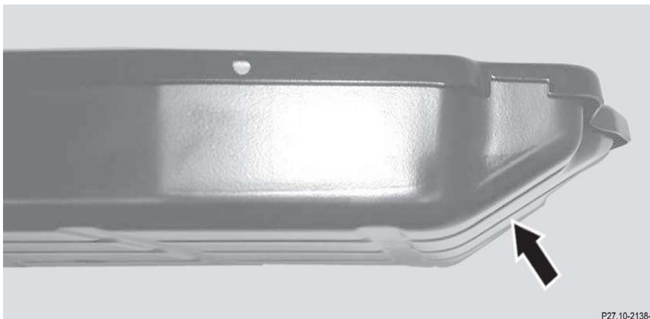
Oil pan (deeper version with slope)
